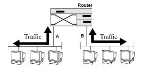
Figure 1-9 Multiple Ethernet Segments Sharing 10 Mbps Bandwidth
